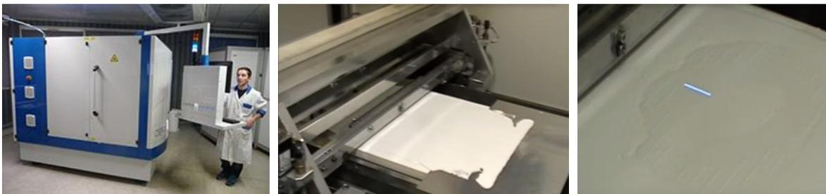
Figure 3: CERAMAKER printer from 3DCer and details of the printing process (doctor blade and laser photo-curing)
